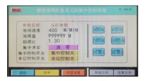
3. Click "Setting Information" in the lower right corner to display the left interface, enter the factory password "123456", and display the right interface
